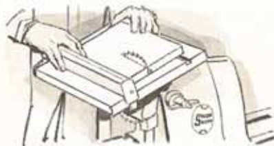
Making a bevel ripping cut with rip fence on tilted table.
