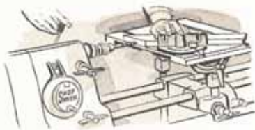
Drilling dowel hole in end of mitered workpiece. Miter gauge set at 45° has positive stop to assure accuracy.
