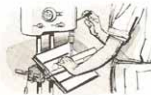
Precise drilling in cylindrical piece with tilting table and fence forming V-block jig.
