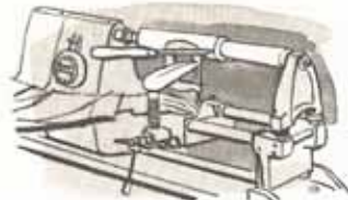
Turning taper with lathe chisel clamped to parallel-traveling tool rest. Adjustable height collars on tailstock assure perfect alignment of centers.
