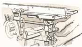
Raising table with rack-and-pinion to exact height calibrated on fence.
