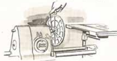
SHOPSMITH converts to a disc sander in seconds with disc that locks on tapered flat of spindle with Allen wrench.
