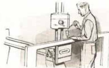
Using SHOPSMITH as floor drill press to mortise hole for door lock. Table adjusted to support workpiece.
