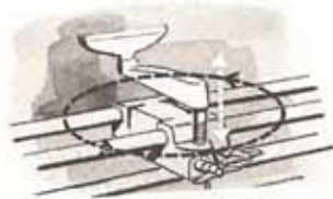
Tool rest always slides parallel to work . . . swings in 360° arc . . . raises or lowers with rack-and-pinion.
