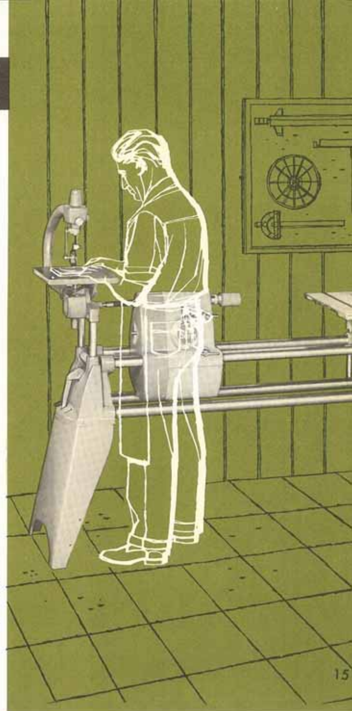
18" MAGNA JIGSAW ON SHOPSMITH. Shown above: Jigsaw on Power Mount, with Drum Sander on front spindle for sanding finished contours of work done on Jigsaw.
