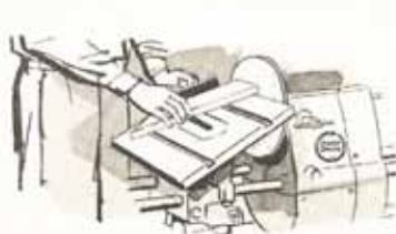
Compound sanding using miter gauge at 45° and table tilted. 45° undercut of table edge and heavily ribbed sanding disc permit chatterless sanding of beveled edges.
