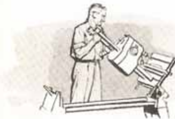
Headrest lock instantly releases headrest for quick, easy change to vertical position.
