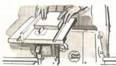
Using SHOPSMITH for molding with Magna Molder accessory mounted on spindle.
