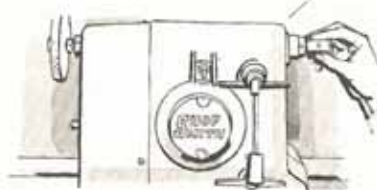
Putting drive center on tapered flat of spindle. Honing wheel on rear auxiliary spindle can be used for sharpening lathe chisels.
