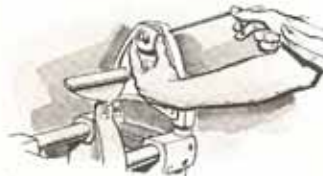
Setting cup center eccentric mount in tailstock with Allen wrench. Eccentric mount offsets cup center up to 1/2" radius for turning tapers.
