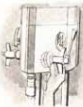
Setting quill feed depth on depth control dial. "Butterfly" handle locks depth control at desired setting.
